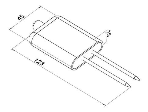
Equipment size drawing (unit: mm)
